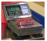
The MCI Solution was to supply the 'Shortie' version of its acclaimed AJA DP Traffic Light Checkscale, with WiFi built in. This is networked with the MCI Myrias Pack Weight Optimising Software with a unique Operator feature. The DP scale displays by number exactly + or— individual fruit need to be added or taken away form the punnet. An error free system. At the same time Myrias in the background runs Average weight optimising correcting scale tolerances in real time to minimise give away
